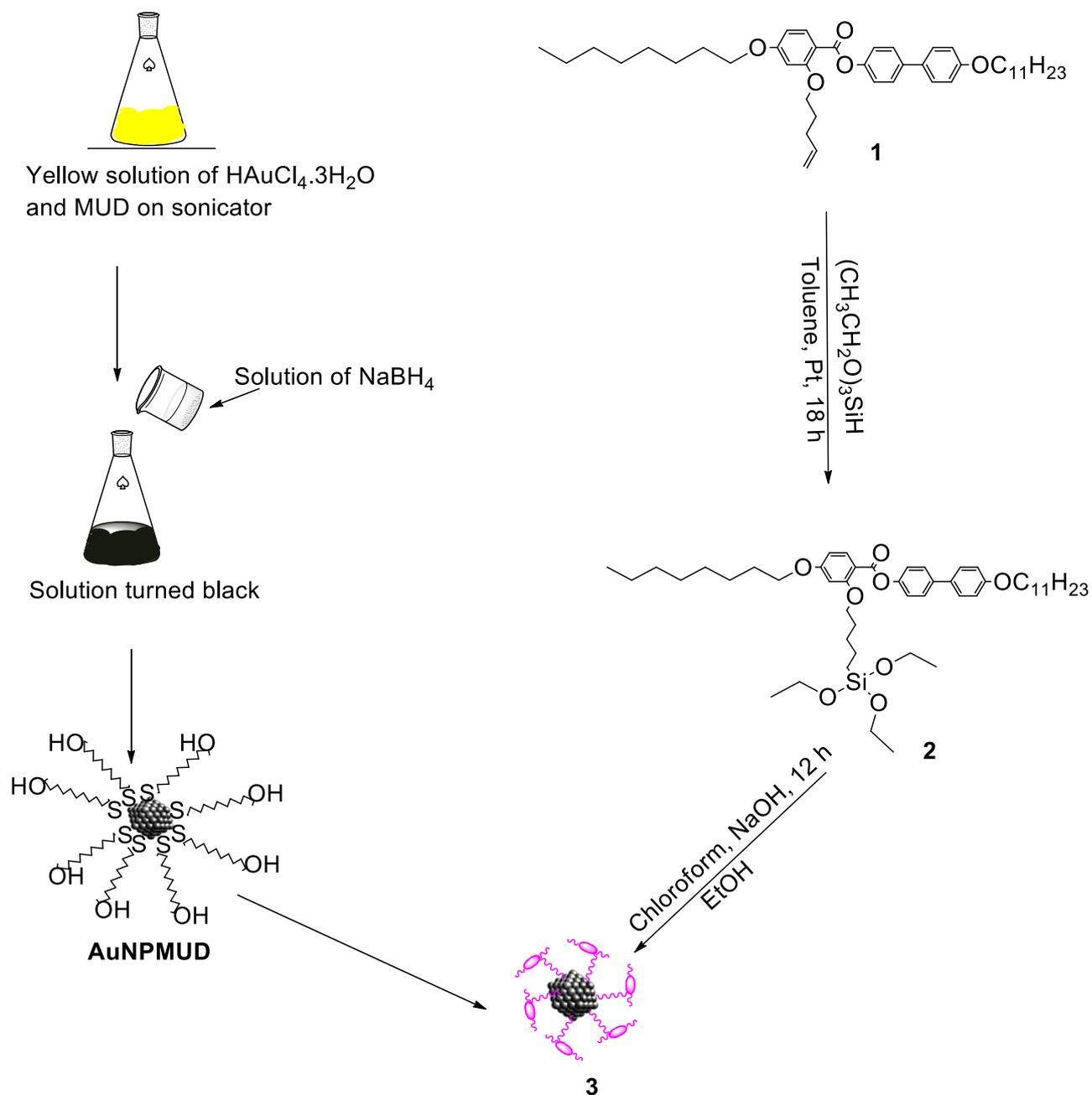
Figure 1: Synthesis of nanocomposite 3.
