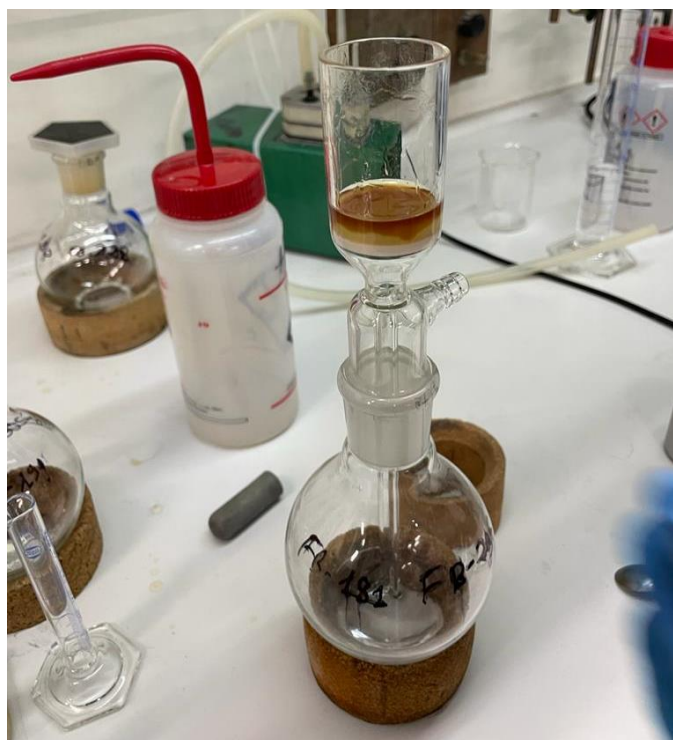
Figure 1. The purification process of a brownish isocyanide on a short silica pad.
