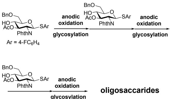
The electrochemical polymerization synthesis of linear oligosaccharides (**2a~8a**) was carried out an H-type divided cell (4G glass filter). The cell had a carbon felt anode (Nippon Carbon JF-20-P7) and platinum square plate (20 mm×20 mm). Building block **1a** (0.200 mmol, 109 mg), Bu<sub>4</sub>NPF<sub>6</sub> (1.00
